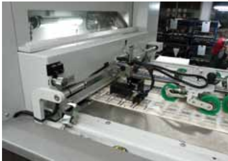
Positiontraverse with camera at the straighten table
